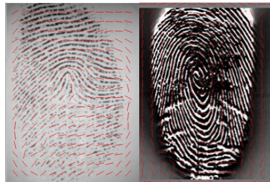
Fig. (5) Estimating ridge orientations of fingerprint images.
