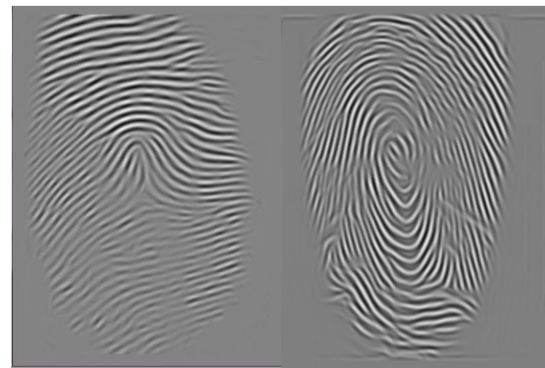
Fig. (6) Applying Gabor filter in order to prepare images for reconstruction
