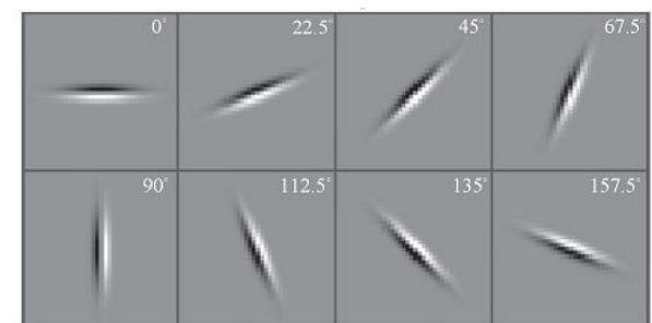
Figure 2- is an anisotropic direction derivative (ANDD) filter in eight directions [12]
